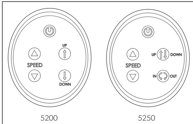
**i** When the fan is running: Closing the lid by using the UP/DOWN button shuts OFF the fan blades. Re-opening the lid by using the UP/DOWN button will revert the fan blade movement to its previous set speed. Using the ON/OFF button will not do this; the ON/OFF button resets the fan to normal operation.
