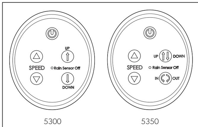
**i** When the fan is running: Closing the lid by pressing the UP/DOWN button shuts OFF the fan blade. Re-opening the lid using the UP/DOWN button will revert the fan blade movement to its previous set speed. Using the ON/OFF button will not do this; the ON/OFF button resets the fan to normal operation.
