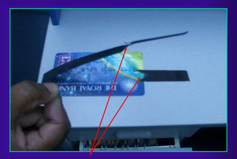
Slits are cut into both sides of the trap, This prevents your card being returned prior to completing your transaction.
