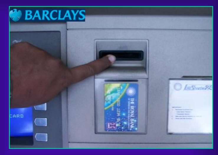
• Once the ends are firmly glued and fixed to the slot, it is almost impossible to detect by unsuspecting clients.
