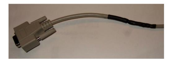
The Elecraft K2 can be controlled from a computer with many popular software packages through the computer's serial port. The K2 requires a custom-made cable to connect the radio to a computer. Under no circumstances can you use a standard serial cable. The K2 manual provides details for building a cable, using a shielded cable and 9-pin "D" connectors (type DB9F).
